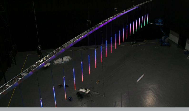
Freeform LED pixel designed for low resolution architectural media facades and shaped displays.
